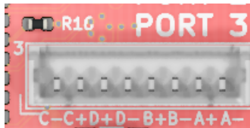
Figure 2: Mapping of ethernet signals onto PicoBlade connectors.
